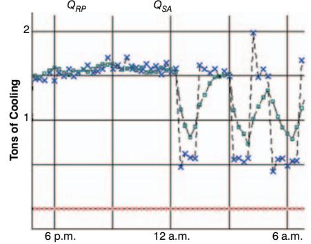
**Figure 7:** Trend plot of DOAS cooling parameters ( $Q_{SA}$ ,  $Q_{RP}$ ) with panel pump on.
