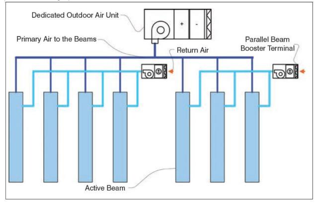
Engineers can pair an ACB system using 100% DOAS supply along with a small quantity of locally recirculated air from *parallel* booster fan/sensible cooling units to increase cooling output during peak load conditions.
